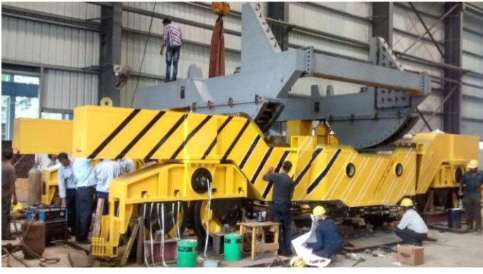
Complete fabrication of Ladle Transfer Car
